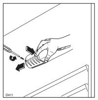
Unscrew the light cover and then pull it outward by pressing as shown in the figure. Unscrew the bulb and replace it with a new 15 watt bulb (available from your nearest Service Force Centre). Replace the light cover by sliding it into its original position and replacing the screw.
